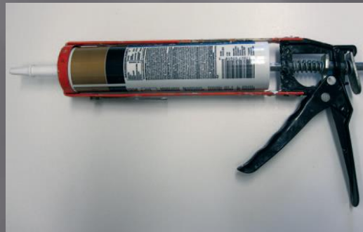
Caulking gun and sealant
