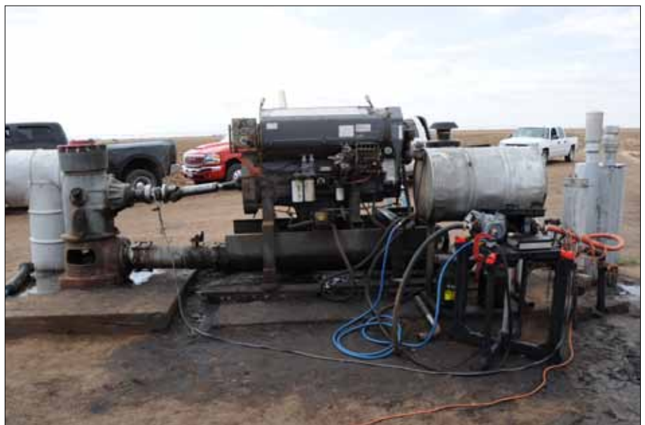
Air cooled Deutz engine on dual fuel. This picture was taken during an evaluation using a torque cell, natural gas meter and diesel flow meter to ideally set fueling mixtures.
