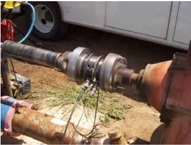
Lebow 1243-20K torque cell in operation. The lines from the torque cell transmit torque and rpm signals to a Daytronics 4K/HP monitor that displays continuous torque, rpm and horsepower readings.
