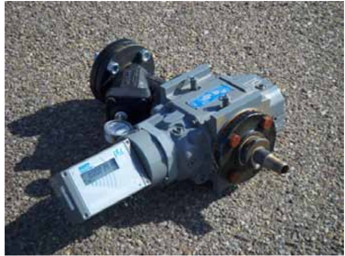
Dresser-Roots Series B rotary gas meter with digital display. This meter is fitted with 1 inch barbed fittings and an inlet filter.
