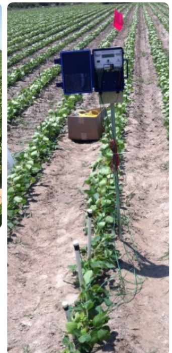
Figure 3. Sensors should be installed early in the season when plants are small so that the installation does not damage roots. Plants with roots that are damaged by sensor installations may not use water the same as undamaged plants.
