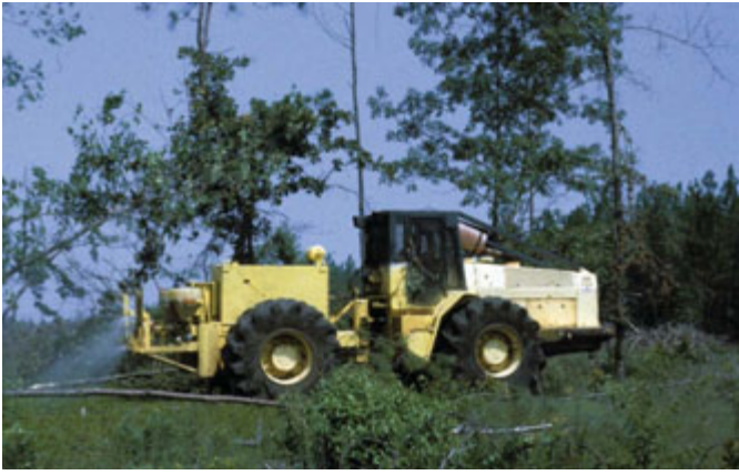
Figure 2. Skidder-mounted spray rig.
