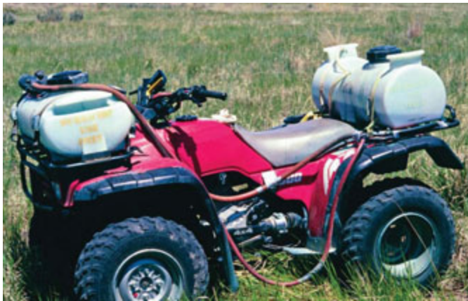
Figure 3. ATV-mounted spray rig.
