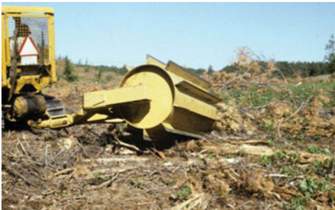
Figure 5. Roller chopping for site preparation.
