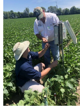
Mississippi Co. Extension agents installing soil moisture sensors.
