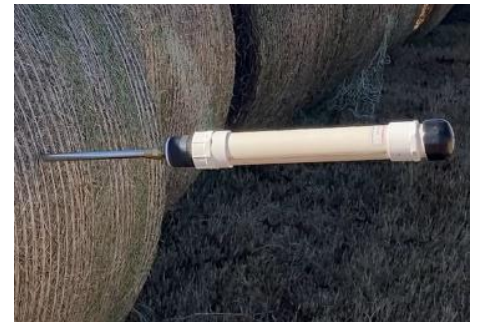
Hay sampler in round hay bale to take core sample for hay quality testing.
