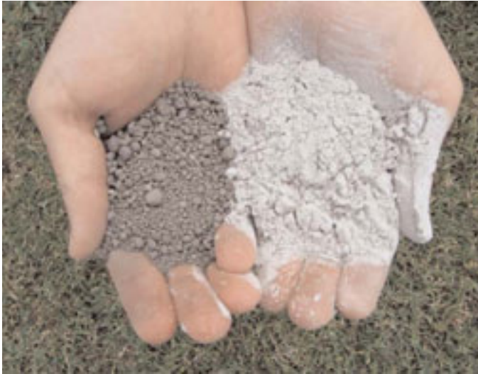
Figure 2. Comparison of pelletized lime (left) and pulverized limestone (right).
